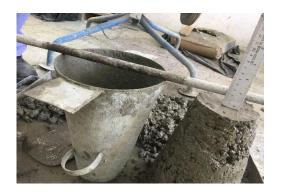
Fig 5: Slump Test
