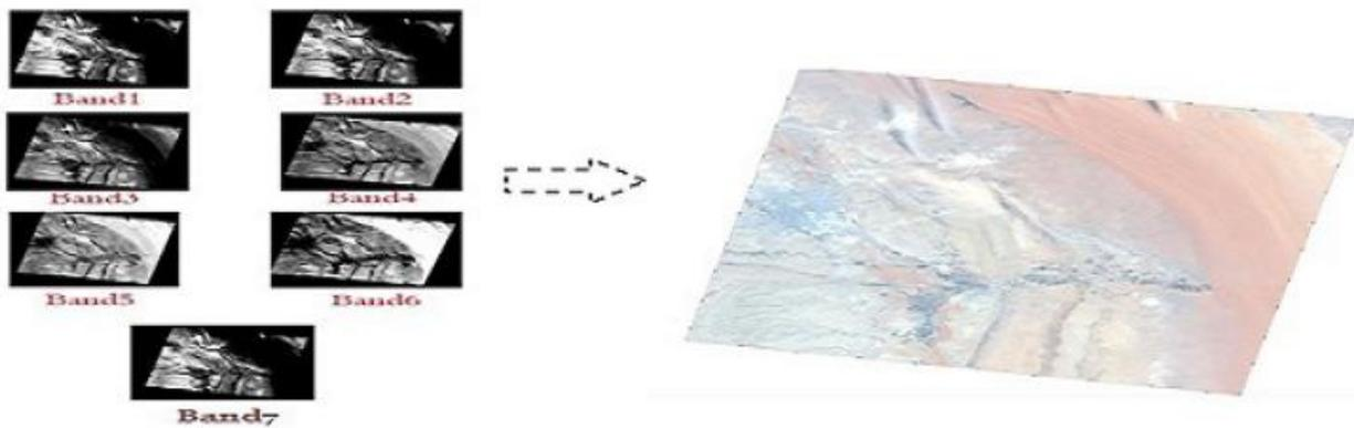
Figure 4: Layer Stacking Proces
